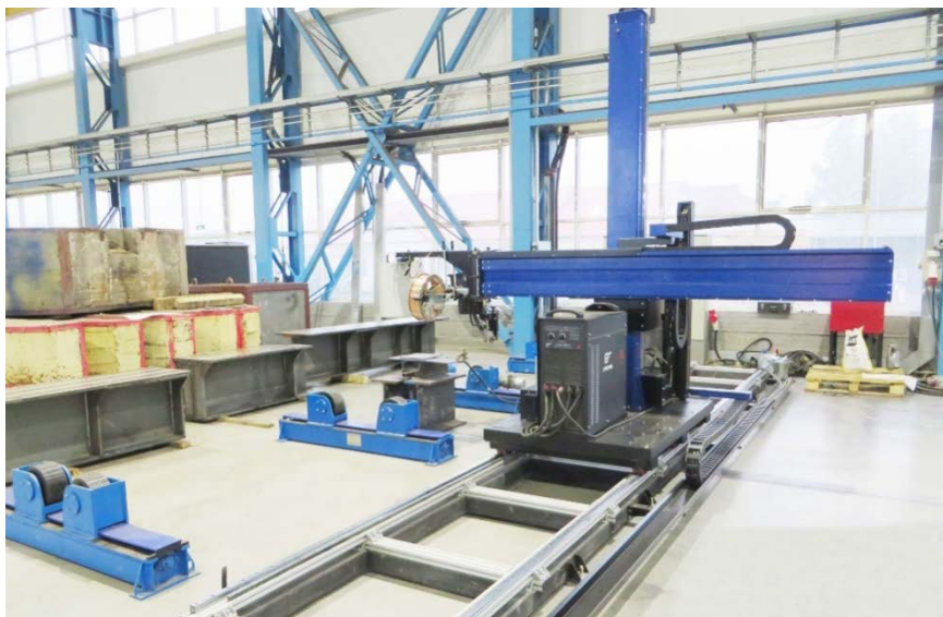
5. Section of the vessel equipment automatic submerged-arc welding
