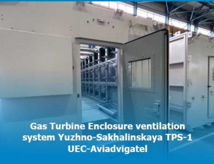
**Gas Turbine Enclosure ventilation system**
